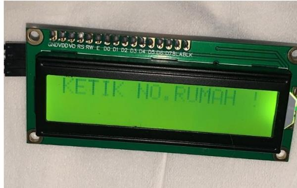
Gambar 2.8 LCD 16x2
